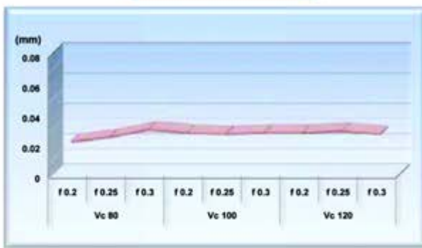
Drilled Hole Size
